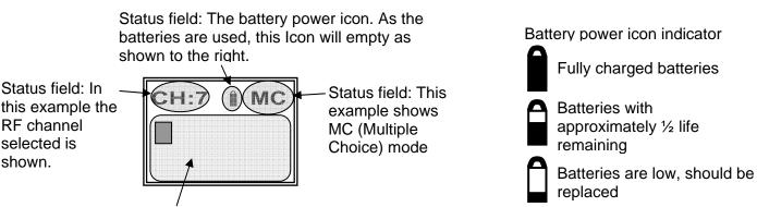
This area of the display is where you would typically input answers. The blinking cursor is a prompt for input. This area has up to 20 characters you can enter and will auto line feed as needed.
